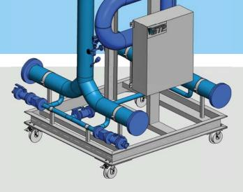
The Prover is a calibrated measuring device that is used for recalibrating on loading facilities. The Prover serves to check flow meters in an on spot loading facility with rail cars filled with light and dark oil products.
